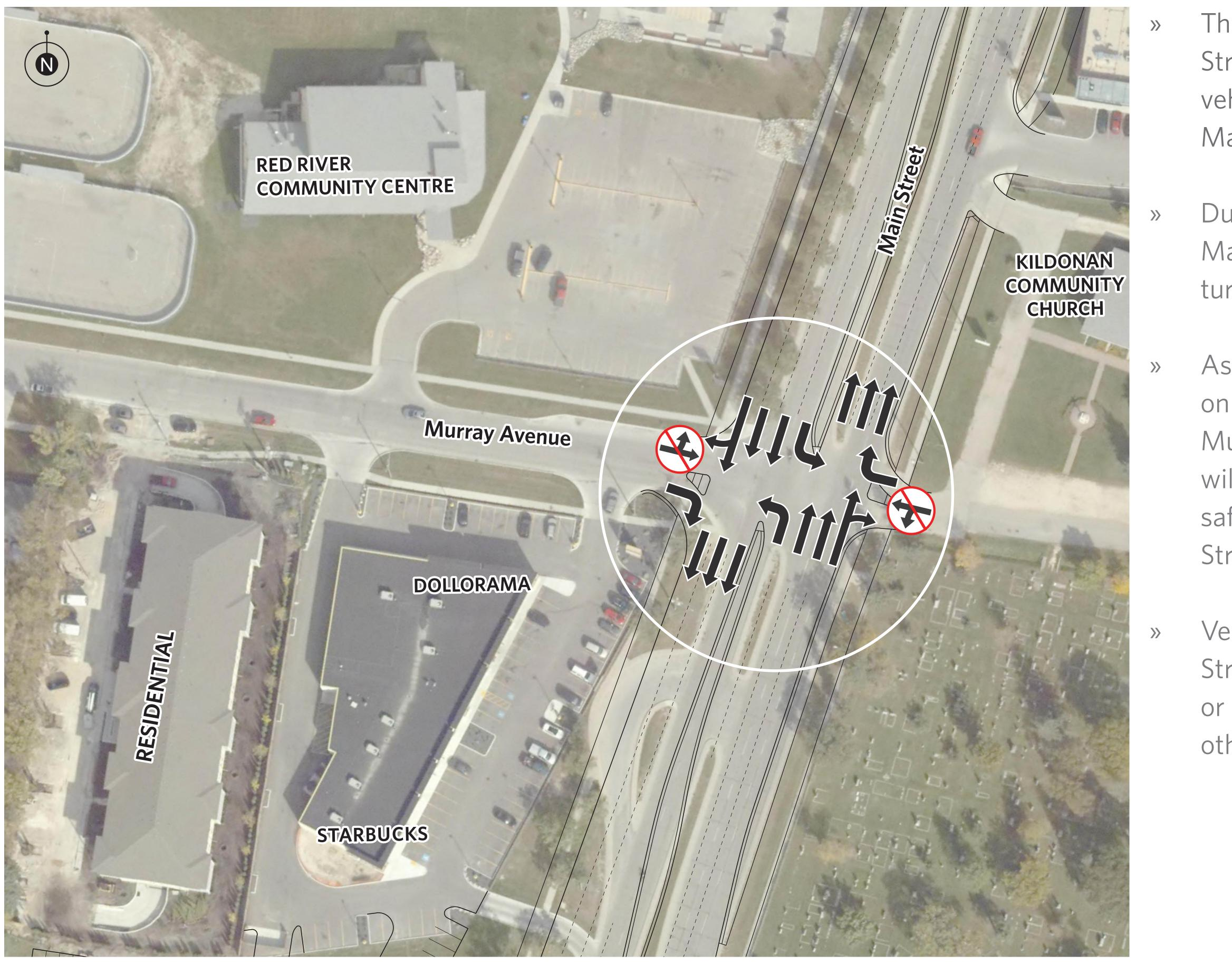
The intersection of Murray Avenue at Main Street has been adjusted to no longer allow vehicles to turn left onto Main Street or cross Main Street.
