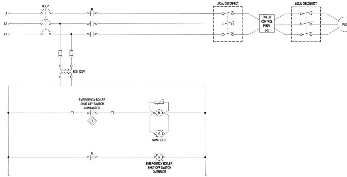
**C** BOILER WIRING SCHEMATIC (WITHIN MCC-1)
