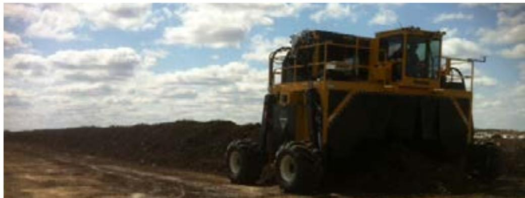
Windrow Turner working on the City's composting pad. Turning yard waste material aids in the compost process. Credit: Solid Waste Services staff.
