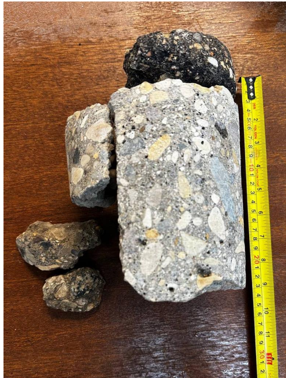
Figure 6. Photos showing Core 6 pavement showing void and deterioration of concrete at joint. Void existed between pavement and base surface
