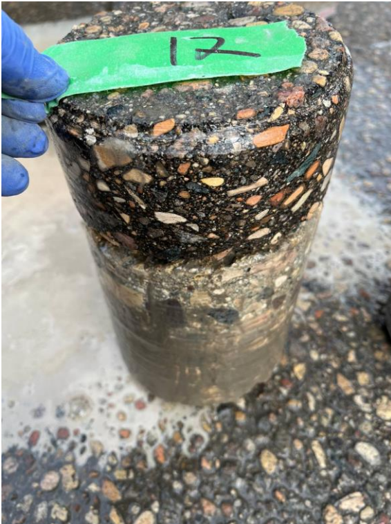
Figure 12. Photos showing Core 12 pavement surface for compressive strength
