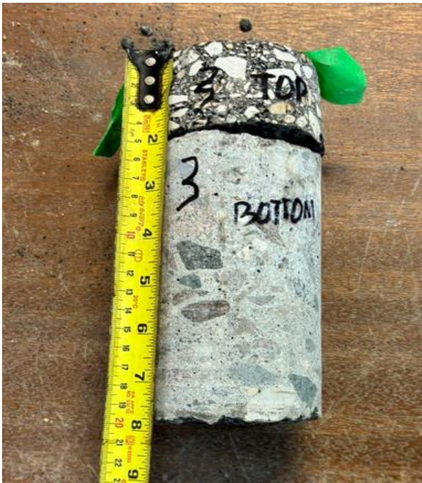
Hartford Ave, WBL, Core 21 (Asphalt Thk 44.5mm, Conc Thk 152.2mm)
