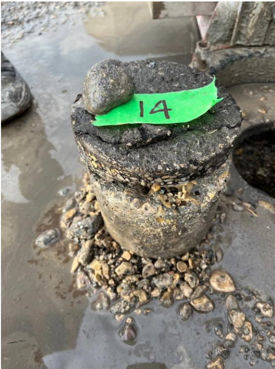
Figure 14. Core 14 showing shear deterioration of concrete and evidence of using cold mix asphalt. Void existed between pavement and base surface
