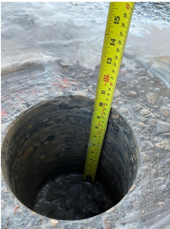
Figure 2. Photos showing Core 2 pavement surface for compressive strength
