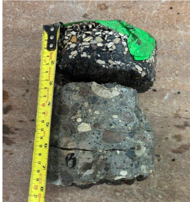
Hartford Ave, EBL, Core 24 (Asphalt Thk 57.2mm, Conc Thk 139.7mm)
