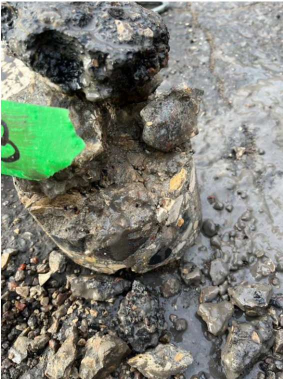
Figure 13. Core 13 showing deterioration of asphalt cold mix was present and concrete presented shear deterioration. Void existed between the pavement and base surface
