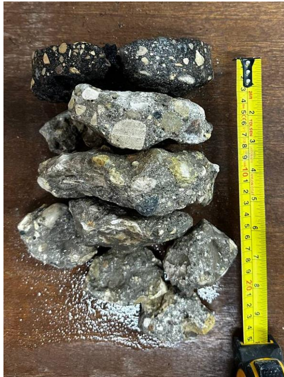
Figure 5. Photos showing Core 5 pavement showing deterioration of concrete and asphalt and void existed between pavement and base surface
