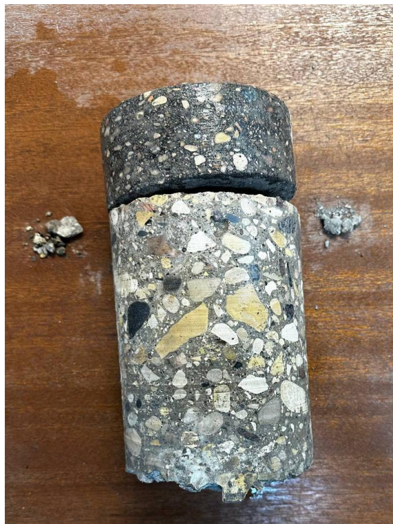
Figure 2. Photos showing Core 2 pavement surface for compressive strength
