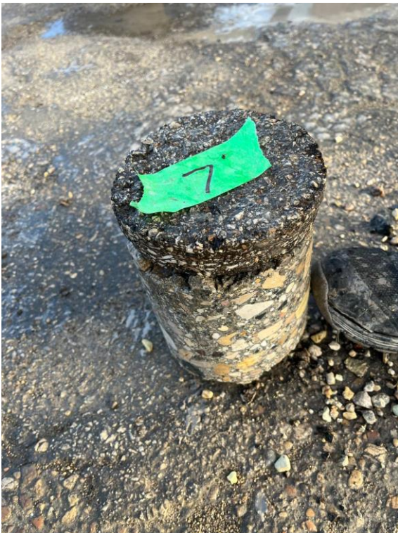
Figure 7. Photos showing Core 7 pavement showing void and gap between asphalt and concrete
