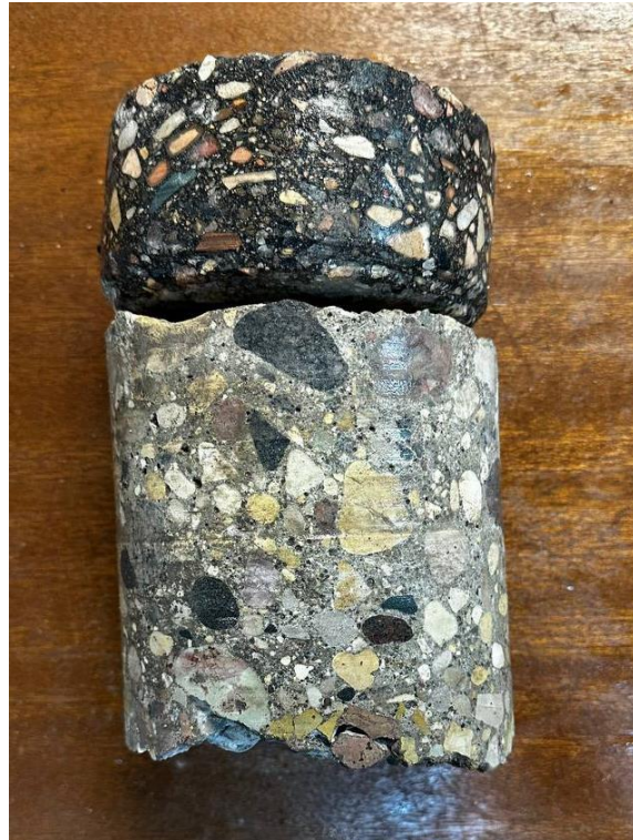
Figure 12. Photos showing Core 12 pavement surface for compressive strength
