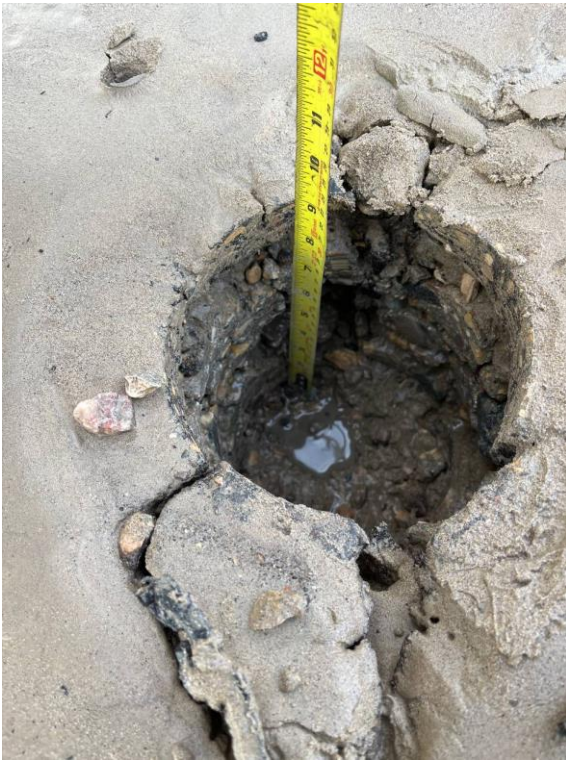
Figure 5. Photos showing Core 5 pavement showing deterioration of concrete and asphalt and void existed between pavement and base surface
