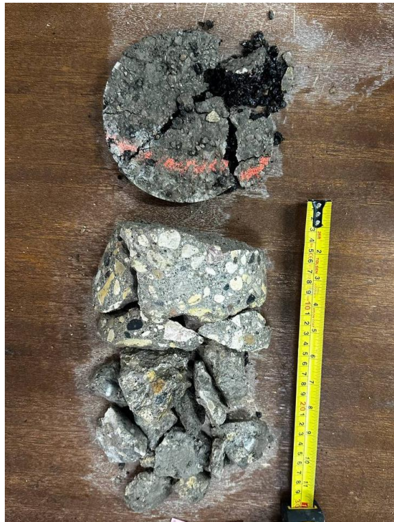
Figure 8. Photo showing Core 8 pavement showing cold mix asphalt and deteriorated concrete. Void existed between the pavement and base surface
