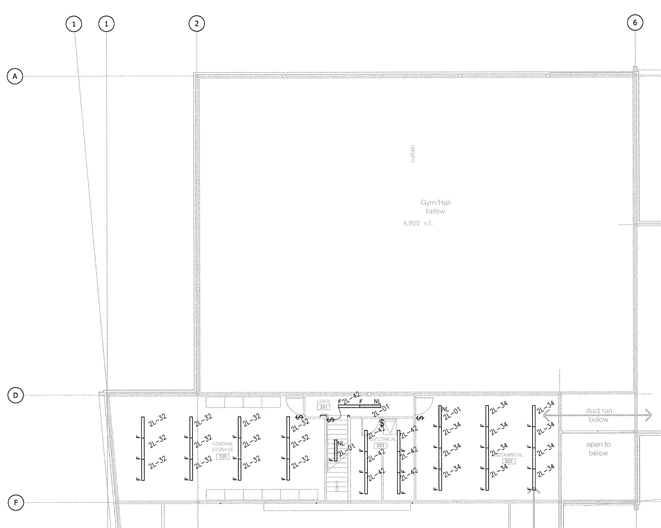
MEZZANINE LIGHTING LAYOUT SCALE: 1:125
