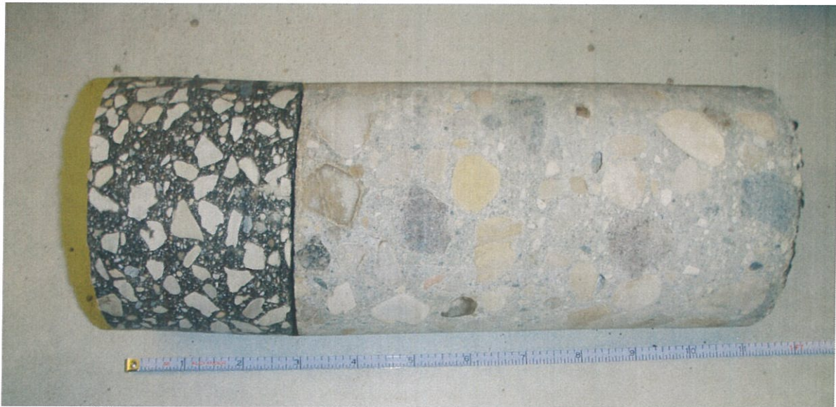
Asphalt and concrete core sample from PH-08-01
