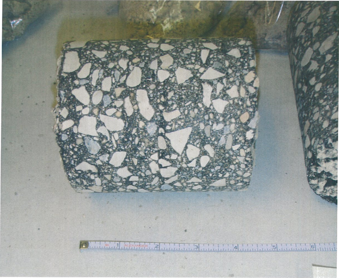
Asphalt core sample from PH-08-05
