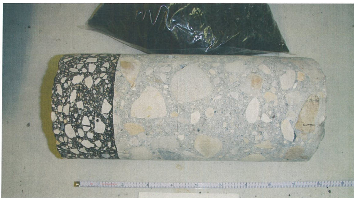
Asphalt and concrete core sample from PH-08-17
