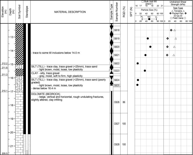
END OF TEST HOLE at 21.6 m in DOLOMITE (BEDROCK) Notes:
