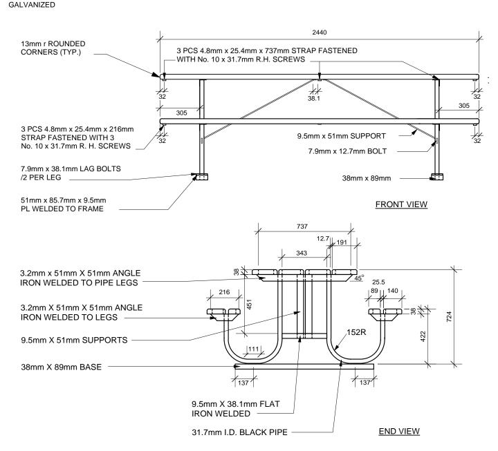
ALL WOOD TO BE FASTENED TO ANGLE IRONS WITH 7.9mm X 38.1mm LAG BOLTS.
