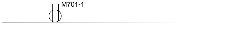
Figure 6-1 : Receptacle Identification on Plan Drawings
