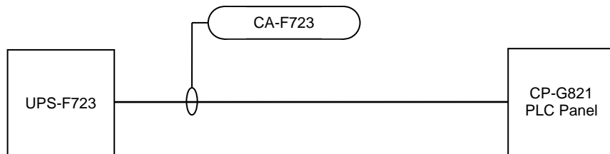
Figure 7-3: Instrument Cable Identification Example – Identified Equipment
