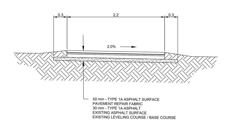
2.0% 50 mm - TYPE 1A ASPHALT SURFACE PAVEMENT REPAIR FABRIC 30 mm - TYPE 1A ASPHALT EXISTING ASPHALT SURFACE EXISTING LEVELING COURSE / BASE COURSE
