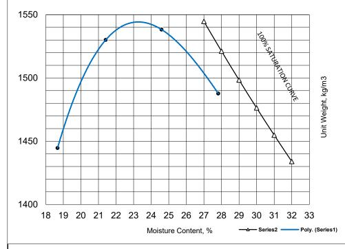
Maximum Dry Density (MDD): 1545 kg/m<sup>3</sup> **Optimum Moisture Content** 23.5 %
