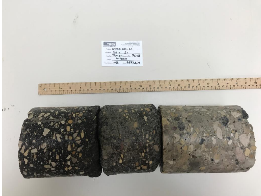
Photo 3: Pavement Core Sample at Test Hole TH19-03
