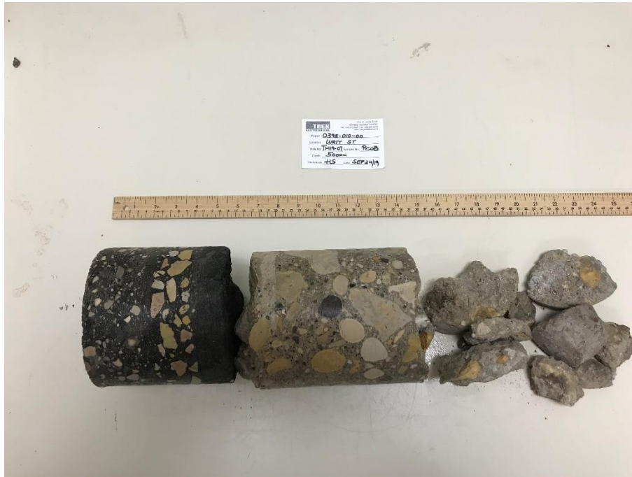
Photo 7: Pavement Core Sample at Test Hole TH19-07
