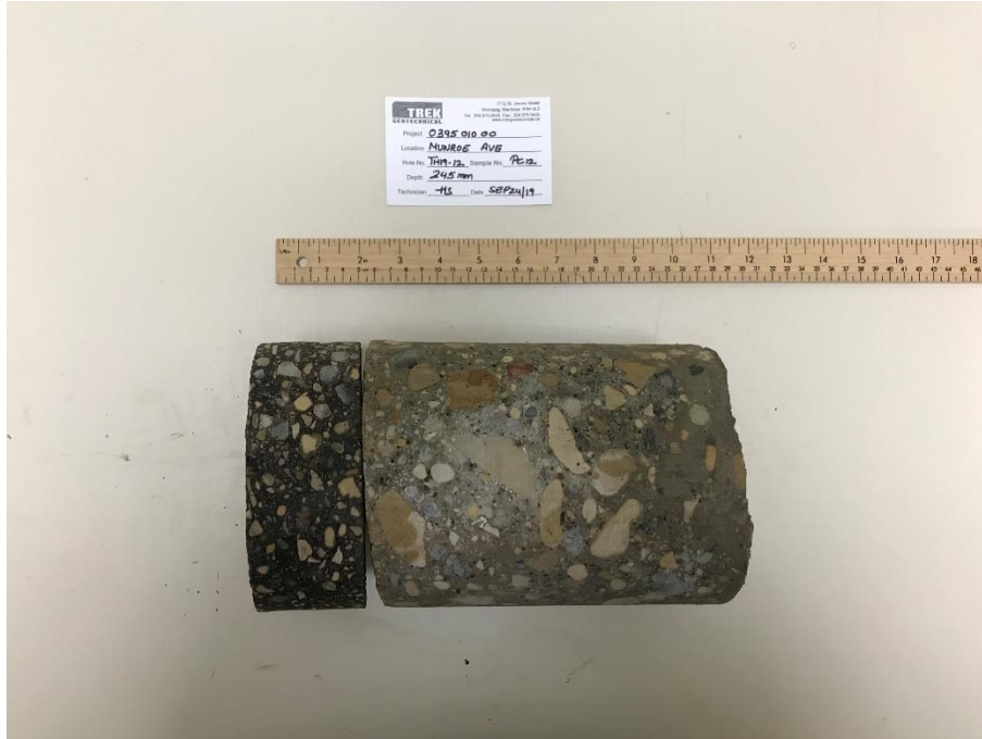
Photo 12: Pavement Core Sample at Test Hole TH19-12
