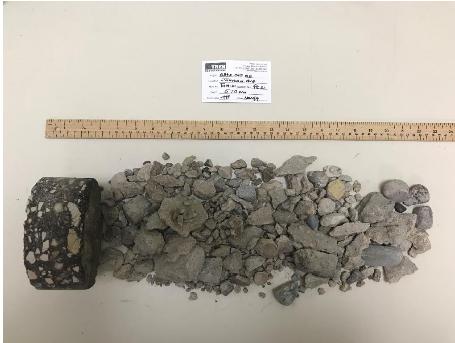
Photo 21: Pavement Core Sample at Test Hole TH19-21
