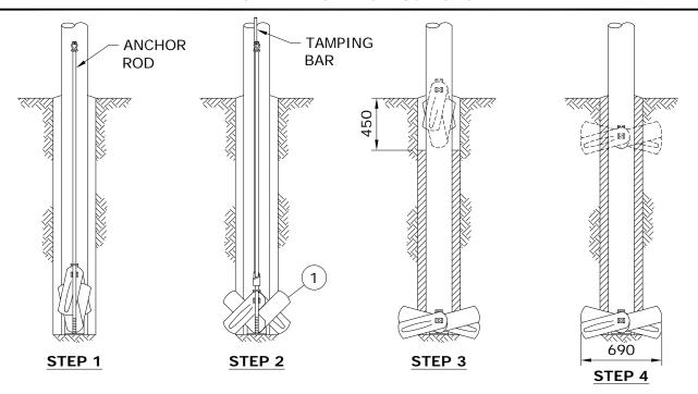
STEP 1: SCREW A 3/4" ANCHOR ROD (NOT INCLUDED WITH ANCHOR) INTO THE POLE KEY AND LOWER THE ASSEMBLY, IN THE CLOSED POSITION, INTO THE HOLE ON THE SIDE OPPOSITE THE STRAIN.
