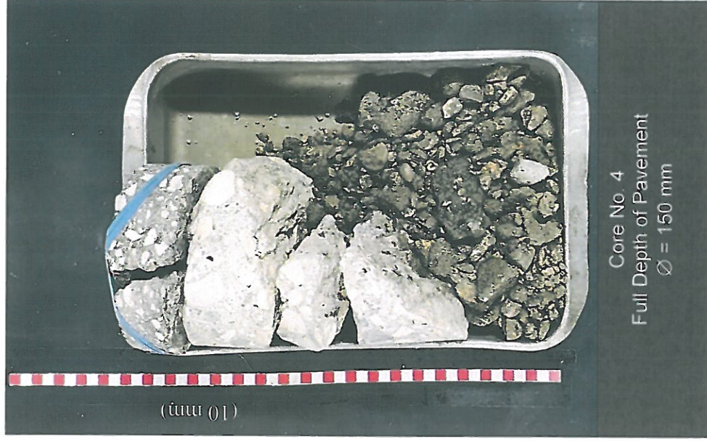
Photograph 4: Specimen from Westbound, Curb Lane
