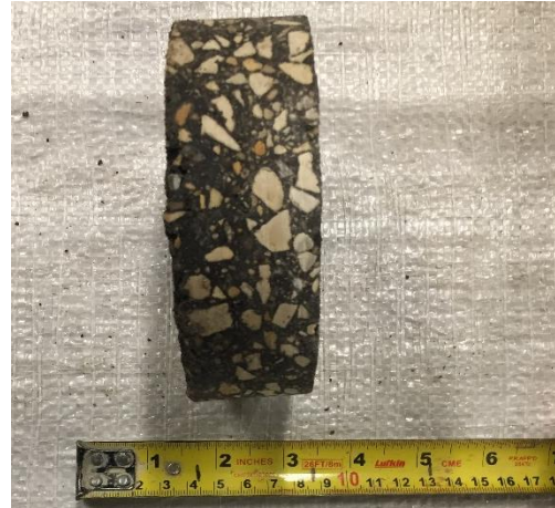
PAN-02: Asphalt Layer, Profile View
