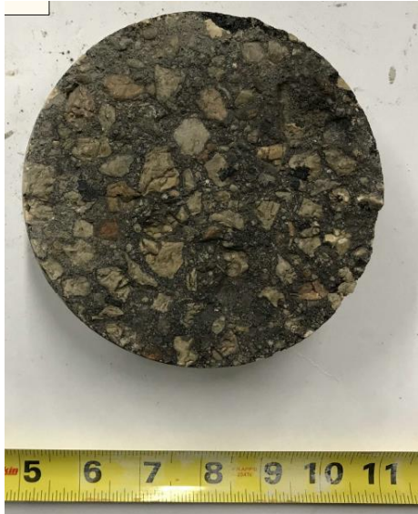
DAY-04: Asphalt Layer, Plan View
