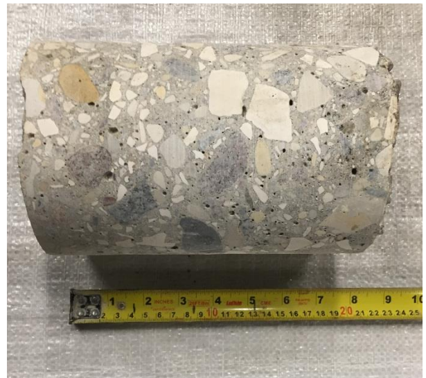
PAN-02: Concrete Layer. Profile View
