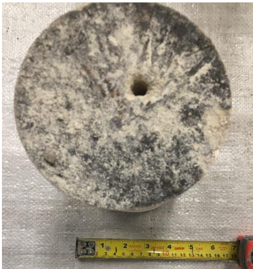
PAN-02: Concrete Layer, Plan View
