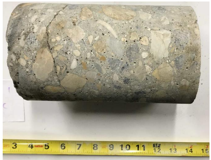
DAY-01: Concrete Layer, Profile View
