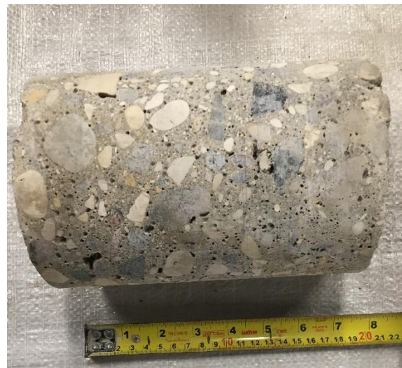
PAN-03: Concrete Layer. Profile View
