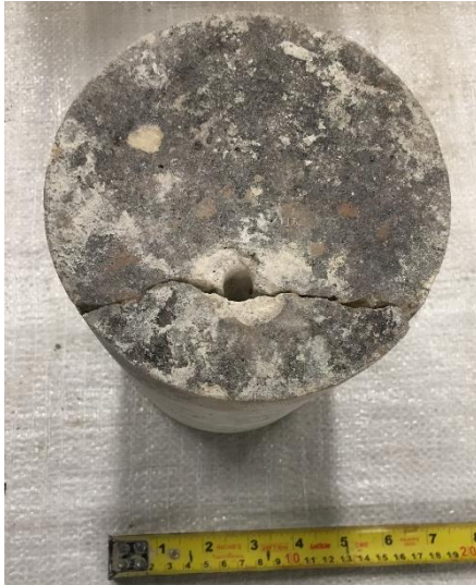
PAN-07: Concrete Layer, Plan View
