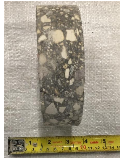
PAN-08: Asphalt Layer, Profile View
