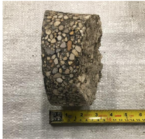
PAN-01: Asphalt Layer, Profile View
