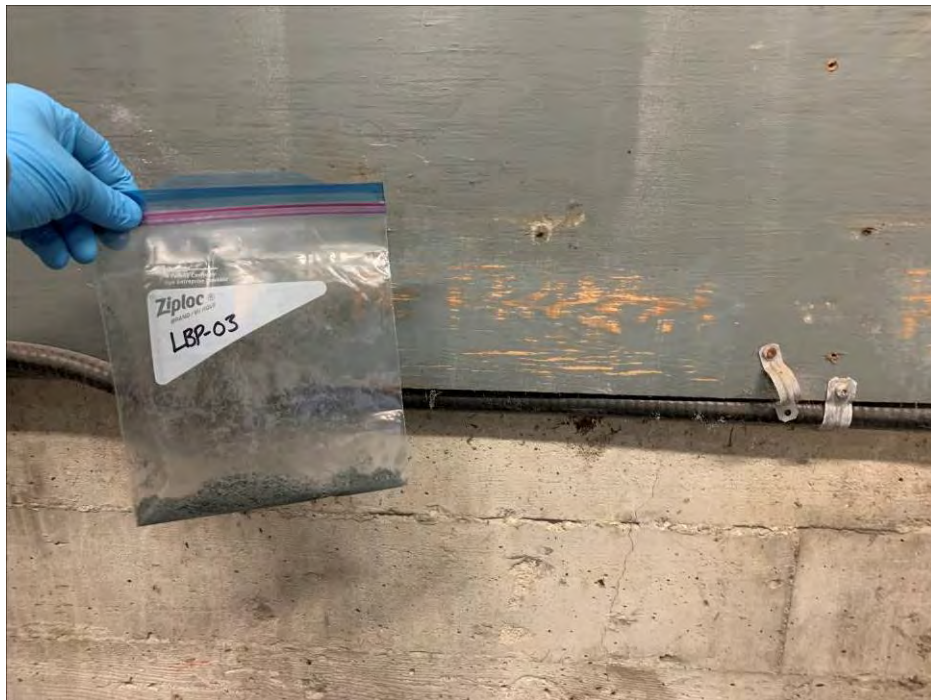
Photo 6: General view of paint chip sample LBP-03 location on the plywood backing board for the electrical panel on the main floor. (April 27, 2021)
