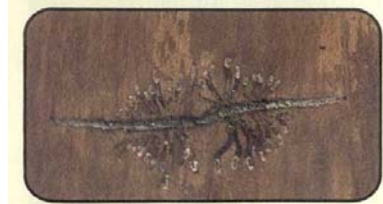
BETLE GALLERY —A beetle gallery is composed of a wide adult tunnel, across the grain of the wood, and many perpendicular larval tunnels. The average length of the adult gallery is 30mm while a larvae gallery may reach 40mm.
